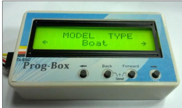
after 1 second, it will enter the first function-MODE TYPE setting interface automatically. Then your esc type can be displayed on the LCD screen. "←" and "→" buttons make no difference because the ESC type can't be changed.
